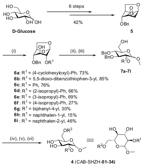
**Scheme 1.** Synthesis of Methyl 6-O-R<sup>2</sup>-2-O-R<sup>1</sup>-D-glucopyranosides CAB-SHZH-01–34. Reagents and conditions: (i) R<sup>1</sup>OH, NaH, EGDME, reflux; (ii) NaH, BnBr, Bu<sub>4</sub>NI, THF, 0 °C to rt; (iii) TMSOCH<sub>3</sub>, TMSOTf, 3 Å MS, CH<sub>3</sub>CN, –45 °C to 45 °C; (iv) TsCl, Et<sub>3</sub>N, DMAP, CH<sub>2</sub>Cl<sub>2</sub>, 0 °C to rt; (v) R<sup>2</sup>OH, NaH, DMF, 80 °C; (vi) Pd/C, H<sub>2</sub>, EtOAc/CH<sub>3</sub>OH = 2:1.
