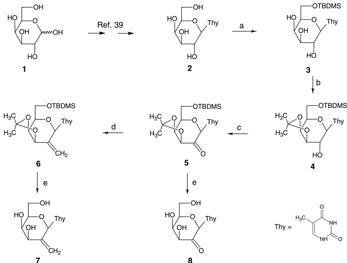
**Scheme 1.** Reagents and conditions: (a) TBDMSCl, pyridine, 0–25 °C, 5 h; (b) acetone, 2,2-dimethoxypropane, *p*-toluenesulfonic acid, 25 °C, 3 h; (c) PDC, Ac<sub>2</sub>O, dry CH<sub>2</sub>Cl<sub>2</sub>, 25 °C, under nitrogen, 4 h; (d) Ph<sub>3</sub>PCH<sub>3</sub>Br, NaH, *t*-amyl alcohol in THF, 0 °C, 2 h, 25 °C, 30 min, under nitrogen; (e) TFA 90% in MeOH, 25 °C, 10 min.
