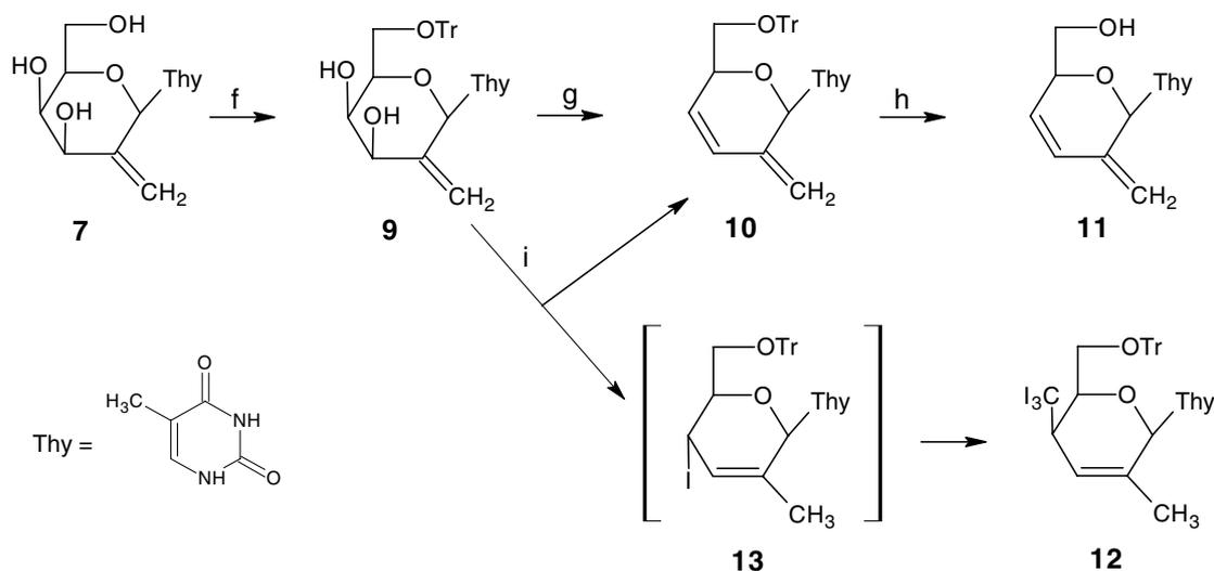
**Scheme 2.** Reagents and conditions: (f) TrCl, pyridine, 25 °C, 4 h; (g) dry Tol/DMF (4:1), iodine–imidazole–Ph<sub>3</sub>P, 100 °C, 1 h; (h) formic acid/diethyl ether, 1:2, 25 °C, 7 min; (i) dry Tol/DMF (4:1), CHI<sub>3</sub>–imidazole–Ph<sub>3</sub>P, 100 °C, 1 h.
