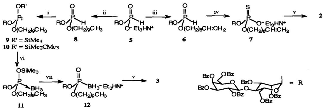
**Scheme 1** Reagents: i, CF<sub>3</sub>CON(SiMe<sub>3</sub>)<sub>2</sub>, THF; ii, *n*-decanol, Me<sub>3</sub>CCOCl, pyridine; iii, dec-9-en-1-ol, Me<sub>3</sub>CCOCl, pyridine; iv, S<sub>8</sub>, toluene-pyridine; v, MeONa, MeOH; vi, BH<sub>3</sub>.THF, THF; vii, 1 M Et<sub>3</sub>NHCO<sub>3</sub> in water (pH 7).
