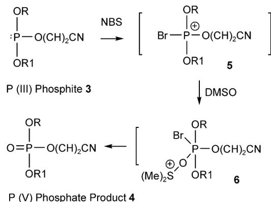
**Scheme 2.** Proposed mechanism for oxidation.
