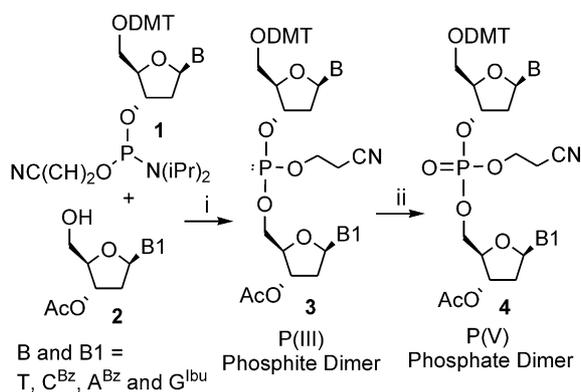
**Scheme 1.** Solution-phase synthesis of 16-dimers. Reagents and conditions: (i) 0.1 mmol **1**, 0.1 mmol **2**,  $\text{CH}_3\text{CN}$ , 1-*H* tetrazole, rt, 2 min, 85–90% **3**; (ii) 0.1 mmol **3**, 6 mL NBS/DMSO/ $\text{CH}_3\text{CN}$  (w/v/v 0.02/0.07/1), rt, 5 min, 90–95% **4**.
