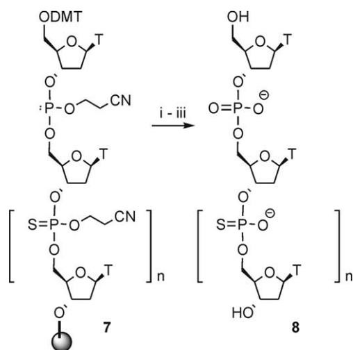
**Scheme 3.** Solid-phase synthesis of tetramer ( $n=2$ ). Reagents and conditions: (i) NBS/DMSO/CH<sub>3</sub>CN (w/v/v 0.04/0.14/1), rt, 2 min, CH<sub>3</sub>CN wash; (ii) detritylation 3% CHCl<sub>2</sub>COOH-CH<sub>2</sub>Cl<sub>2</sub>, 1.8 min; (iii) NH<sub>4</sub>OH 55 °C.
