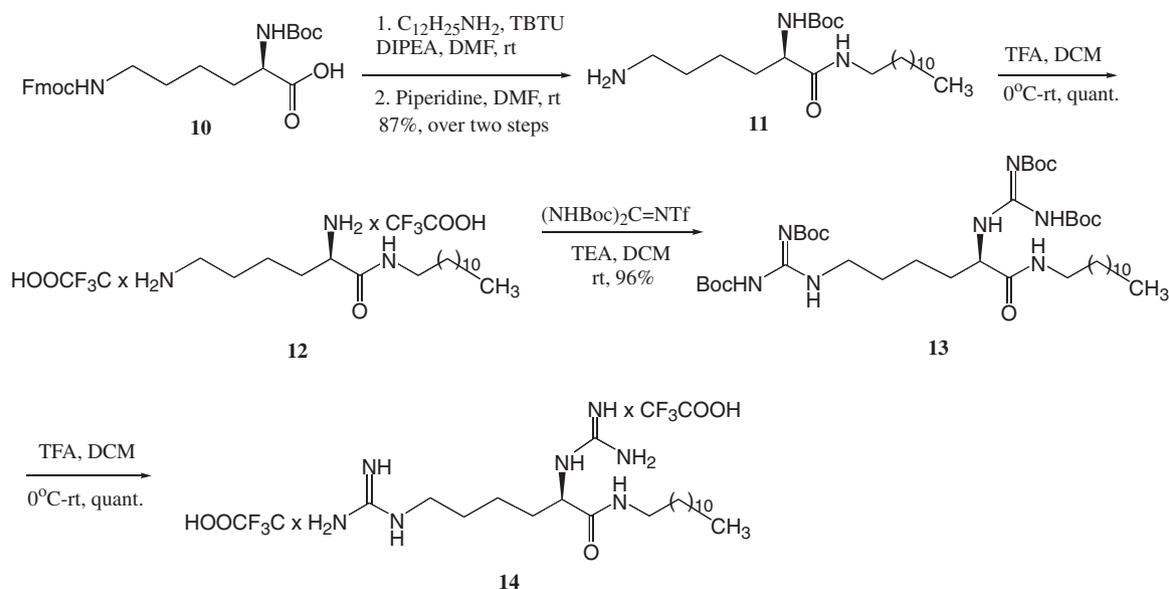
**Scheme 3.** Synthesis of lysine- (**12**) and guanidinylated lysine-based (**14**) reference lipids.
