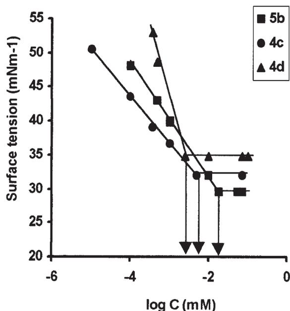
**Fig. 2.** Plots of interfacial tension (obtained by tensiometry) vs. log [bolaform] at 25°C in water.
