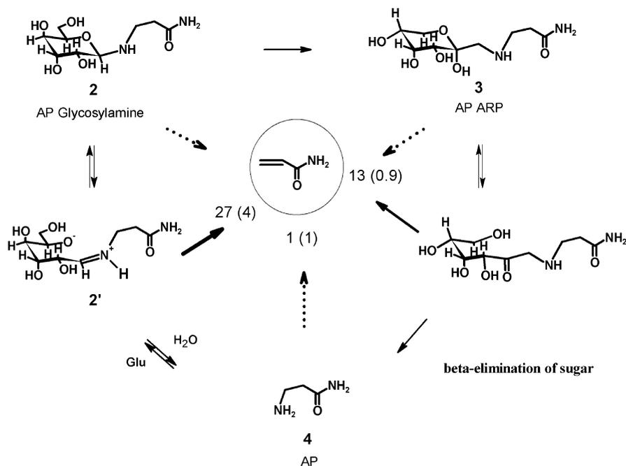
**Figure 4.** Reactive precursors and their relative abilities to generate acrylamide in wet and dry (values in parentheses) model systems (see also **Table 2**). Glu, glucose; AP, 3-aminopropionamide; ARP, Amadori rearrangement product.
