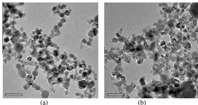
**Figure 2.** TEM images of (a) native CuO nanoparticles, (b) CuO nanoparticles after three cycles.
