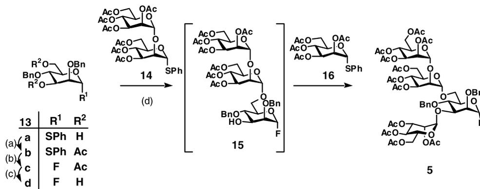
Scheme 2. Reagents and conditions: (a) Ac<sub>2</sub>O, pyridine, rt, 7 h. (b) NBS, DAST, CH<sub>2</sub>Cl<sub>2</sub>, -10 °C, 12 h. (c) NaOMe, MeOH, 0 °C, 4 h, 77% (three steps). (d) NIS, TfOH, 4A MS, CH<sub>2</sub>Cl<sub>2</sub>, -40 °C, 1 h, then **16**, -40 °C, 0.5 h, 48% (+21% pentasaccharide).
