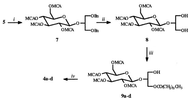
**Scheme 2.** Reagents: (i)  $(\text{ClCH}_2\text{CO})_2\text{O}$ ,  $\text{CH}_2\text{Cl}_2/\text{Py}$ , 0°C; (ii)  $\text{H}_2$ , Pd/C; (iii) LCA,  $\text{CF}_3\text{CH}_2\text{OCO}(\text{CH}_2)_n\text{CH}_3$ , THF; (iv)  $\text{NH}_2\text{NH}_2\cdot\text{AcOH}$ ,  $\text{AcOEt}/\text{MeOH}$ ; MCA =  $\text{COCH}_2\text{Cl}$ .
