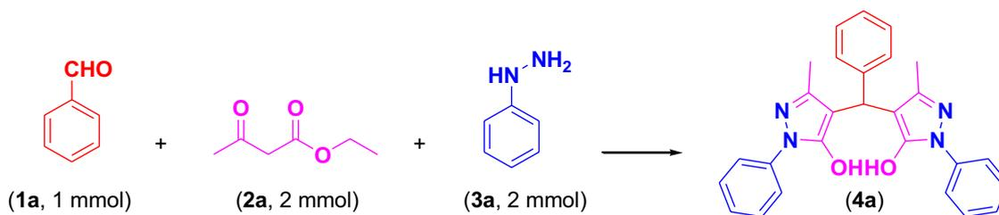
**Scheme 3** The one-pot condensation of benzaldehyde (**1a**) (1 mmol, 0.10 g), ethyl acetoacetate (**2a**) (2 mmol, 0.26 g) and phenylhydrazine (**3a**) (2 mmol, 0.21) in the presence of ((SB-DABCO)HSO<sub>4</sub>)
