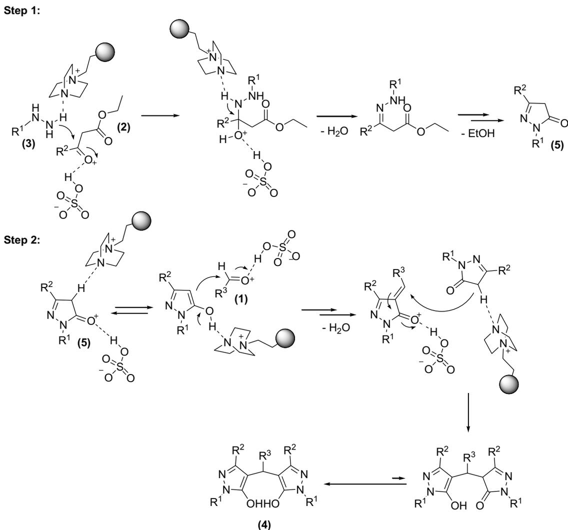
**Scheme 5** The proposed mechanism for the synthesis of bis(pyrazolyl)methanes in the presence of ((SB-DABCO)HSO<sub>4</sub>)
