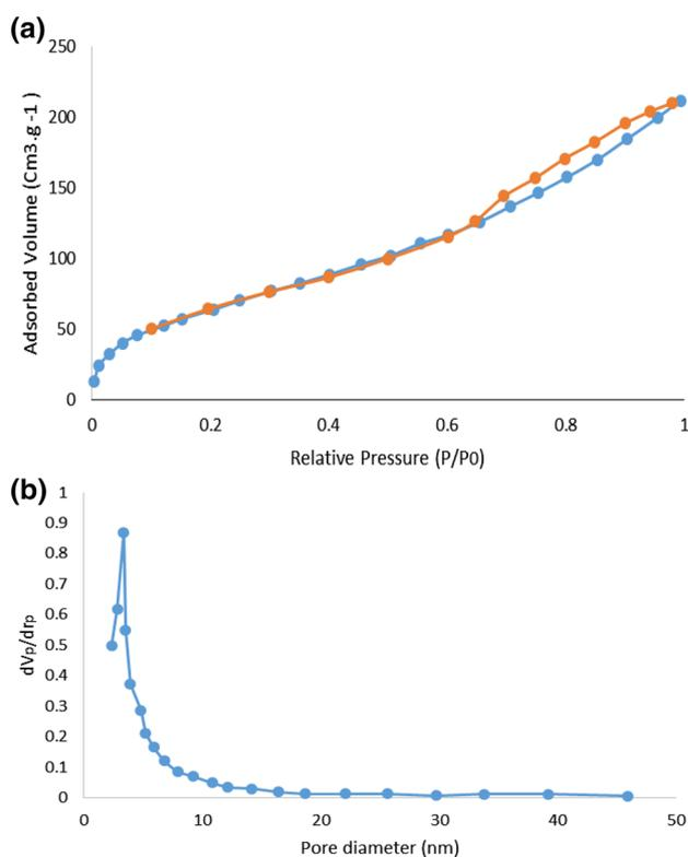
**Fig. 4** The nitrogen adsorption–desorption isotherms (a) and the pore size distribution (b) of (SB-DABCO)HSO<sub>4</sub>
