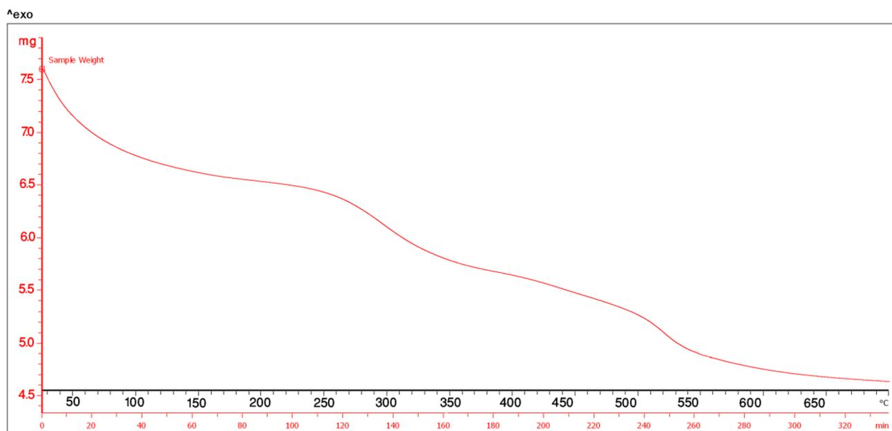
**Fig. 2** The TG analysis of silica-bonded *n*-propyl-4-aza-1-azoniabicyclo[2.2.2]octane hydrogen sulfate ((SB-DABCO)HSO<sub>4</sub>)
