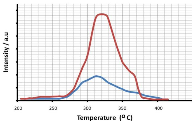
**Fig. 3** The CO<sub>2</sub>-TPD plots of SiPrCl (blue) and (SB-DABCO)HSO<sub>4</sub> (red)
