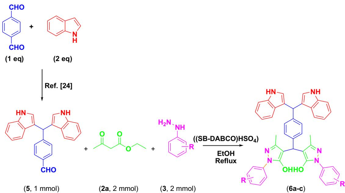
**Scheme 4** The synthesis of some novel 4-[bis(pyrazolyl)methane]phenylmethylene-bis(indole)s in the presence of ((SB-DABCO)HSO<sub>4</sub>)
