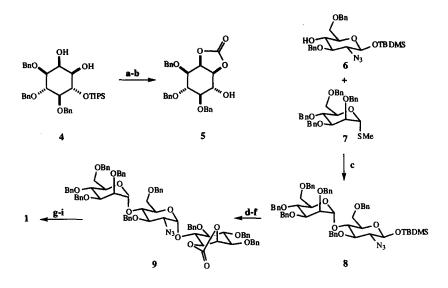
(a) N, N'-carbonyldiimidazole, benzene, 20 °C, 17h; (b) TBAF, THF, 0 °C, 3 min (84% over 2 steps); (c) PhSeCl, AgOTf, toluene, - 42 °C, 1 h (53%); (d) *n*-BuN<sub>4</sub>F, HOAc, THF, 20 °C (84%); (e) DAST, THF, -42 °C, 30 min (90%); (f) 5, Cp<sub>2</sub>ZrCl<sub>2</sub>, AgOTf, toluene, -42 °C to 20 °C, 5h (28%  $\alpha$ ; 26%  $\beta$ ); (g) 1 M LiOH, THF, 20 °C, 12h, (80%); (h) MeOPOCl<sub>2</sub>, pyridine; (i) Na, NH<sub>3</sub> (l), -78 °C, 15 min (56% over 2 steps).
