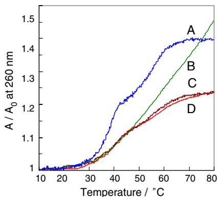
**Figure 4.** Melting curves of nucleo-cages; (A) unmodified nucleo-cages, (B–D) Lac-NCs (concentration of **4** for photo-crosslinking: (B) 600  $\mu$ M, (C) 450  $\mu$ M, (D) 300  $\mu$ M).
