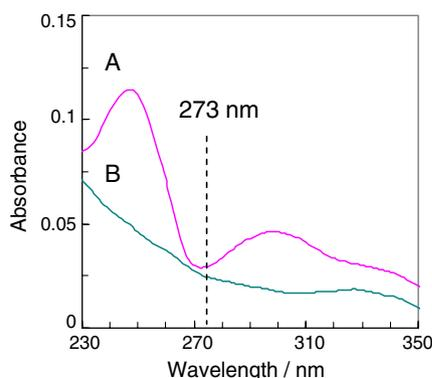
**Figure 3.** UV-vis spectra of ultrafiltration filtrate of nucleo-cages aqueous solutions at 25 °C. (A) Before and (B) after UV irradiation in the presence of **4** (300  $\mu$ M).
