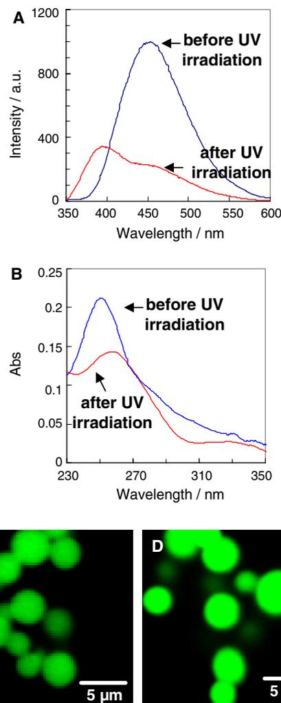
**Figure 2.** (A) Fluorescence spectra ( $\lambda_{\text{ex}}$ , 330 nm) and (B) UV-vis spectra of nucleo-cages aqueous mixtures before and after UV irradiation. CLSM images of (C) unmodified nucleo-cages and (D) Lac-NCs ( $[\mathbf{4}] = 300 \mu\text{M}$ ;  $[\text{ODN}]_{\text{total}} = 20 \mu\text{M}$ ,  $[\text{NaCl}] = 0.5 \text{ M}$ ,  $[\text{YOYO-1}] = 1 \mu\text{M}$  at  $10^\circ\text{C}$ ).
