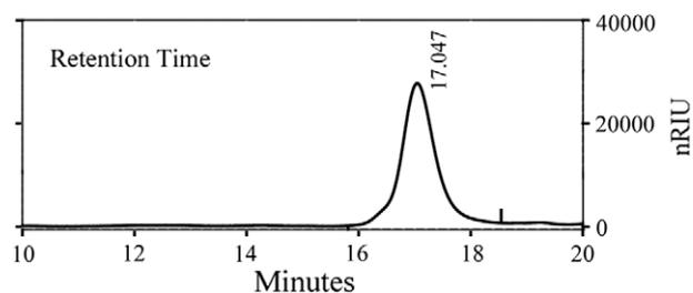
**Figure 4.** GPC chromatogram of polymer products generated in condition No. 8 of Table 1.
