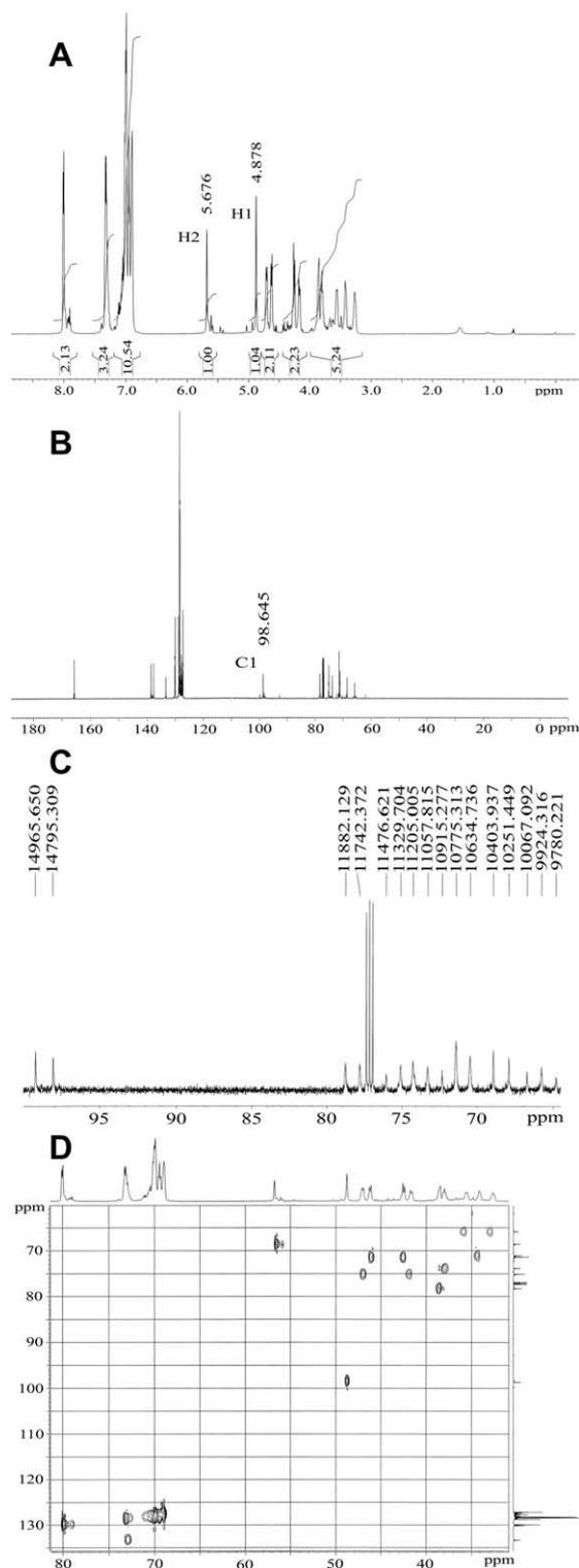
**Figure 3.** NMR spectra of polymer products generated in condition no. 8 of Table 1: (A)  $^1\text{H}$  NMR, (B)  $^{13}\text{C}$  NMR, (C)  $^{13}\text{C}$ – $^1\text{H}$  coupled  $^{13}\text{C}$  NMR, and (D) HMQC 2D NMR.
