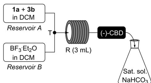
Figure 2. General apparatus for the flow synthesis (-)-CBD.
