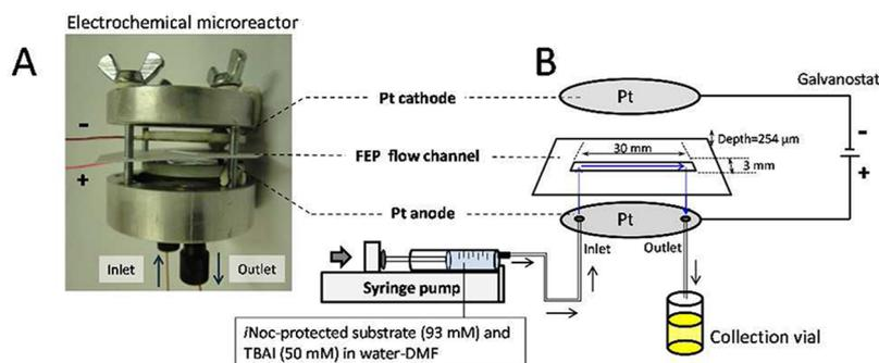
Figure 2. (A) Electrochemical microreactor device (opened). (B) Flow setup for the electrochemical deprotection of the *iNoc* group.
