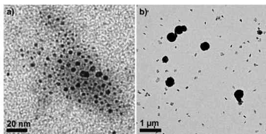
**Figure 1.** TEM images of the prepared palladium nanoparticles: (a) Pd@1\* and (b) Pd@2\*.
