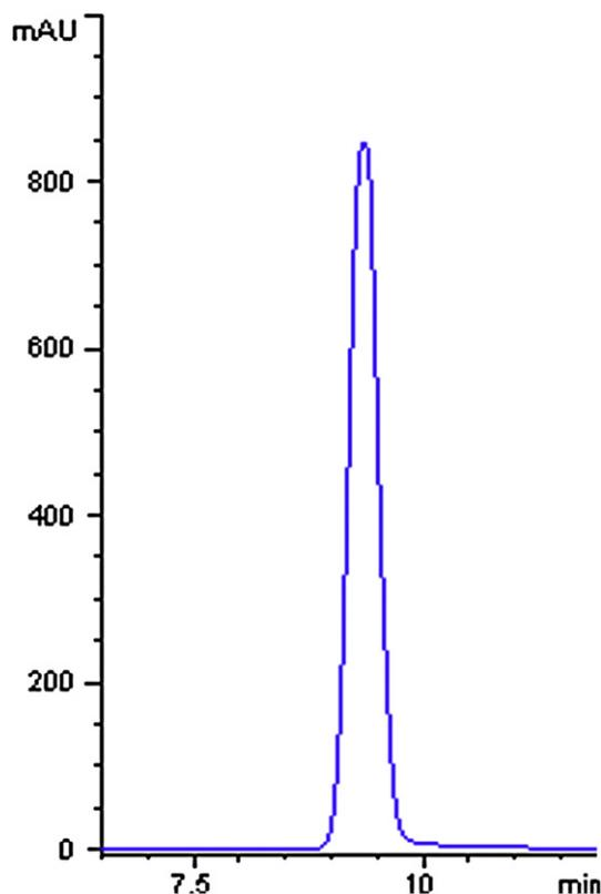
**Fig. 4.** HPLC chromatogram of the target compound **IIf**. Only one isomer was found at the retention time of 9.374 min.
