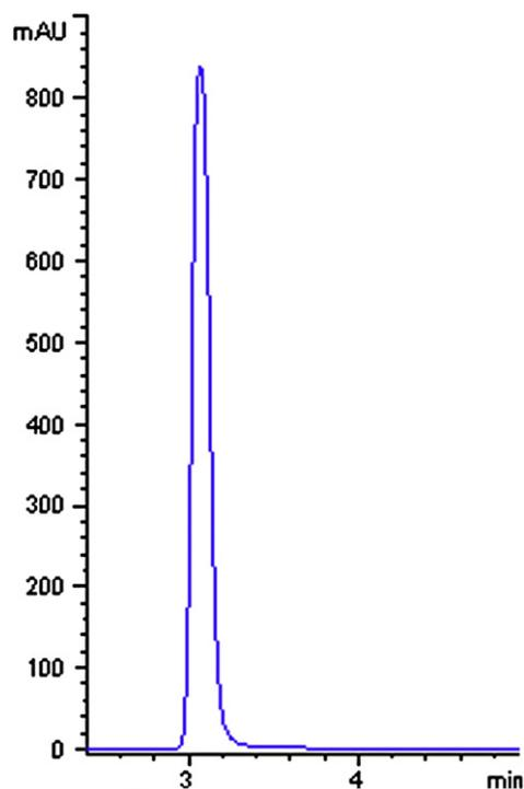
**Fig. 3.** HPLC chromatogram of the target compound **If**. Only one isomer was found at the retention time of 3.068 min.
