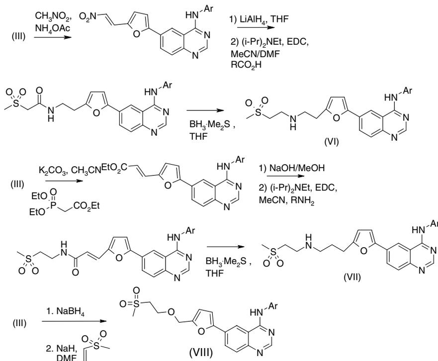
**Scheme 4.** Synthesis of furan side-chain substitutions on the 4-anilinoquinazoline scaffold.
