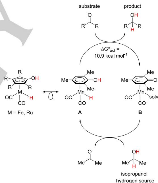
**Scheme 1.** Initially proposed mechanism for the hydrogen transfer by manganese phenol complex.
