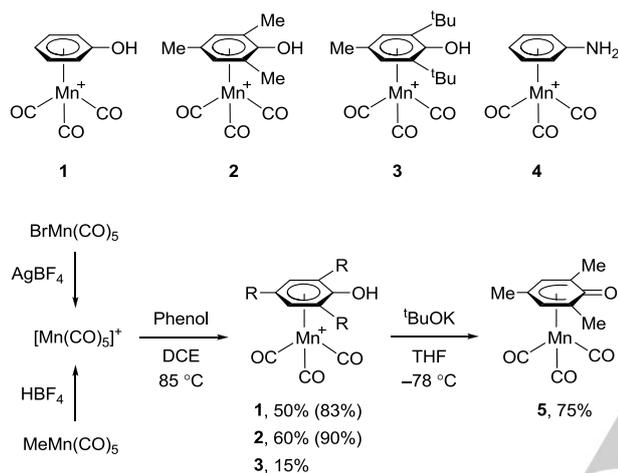
**Scheme 2.** Synthesis of manganese catalysts. Cationic complexes were isolated as salts with BF<sub>4</sub><sup>-</sup> counter-ions, which are omitted on the scheme. Yields in parentheses refer to the synthesis from MeMn(CO)<sub>5</sub>.
