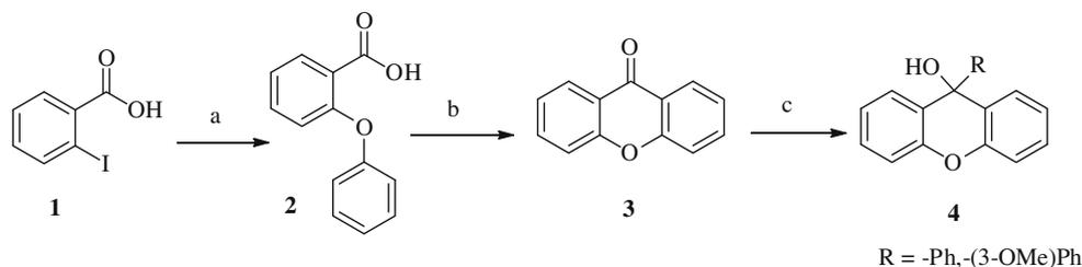
Scheme 1. Synthesis of the 9-alkylxanthen-9-ols. Reagents and conditions: (a) phenol, Cu, CuI, pyridine, DBU, DMF, reflux; (b) H<sub>2</sub>SO<sub>4</sub>, 100 °C; (c) MgBrR, THF, –78 °C 1 h to rt 5 h.
