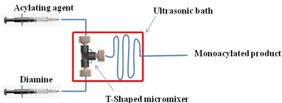
**Figure 1.** Length of capillary microreactor dipped in ultrasonic bath(330W) = 50 cm (effective volume = 0.098 ml); length of capillary microreactor outside ultrasonic bath = 10 cm
