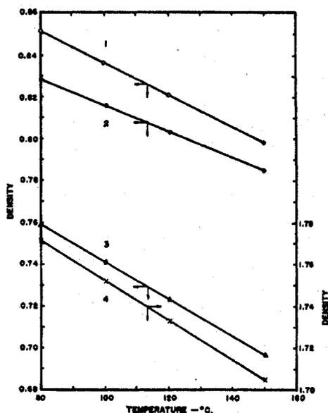
Figure 1. Variation of Density with Temperature
