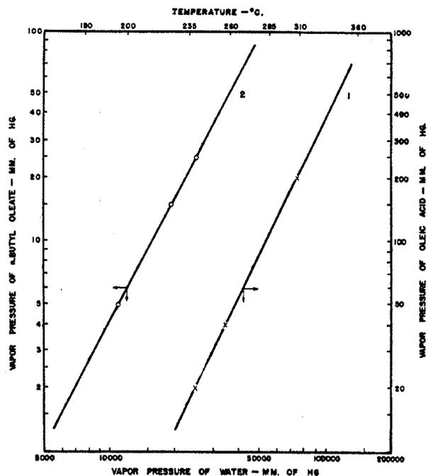
Figure 13. Correlation of Data against Vapor Pressure of Water
