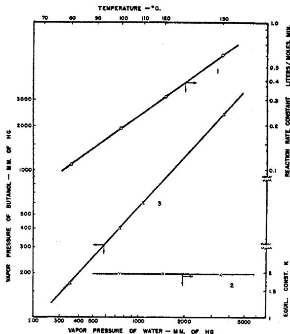
Figure 12. Correlation of Data against Vapor Pressure of Water
