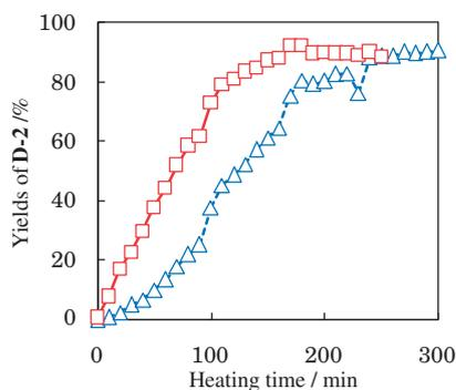
**Figure 2.** The formation of **D-2** from **2a** as a function of heating time in the presence (red) and absence (blue) of 13 mM piperidine in methanol- $d_4$  at 100 °C.
