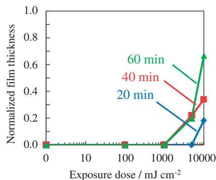
**Figure 5.** Photosensitivity curves of PGMA films containing 7.4 mol % of **1a** (toward epoxy groups) and 2.2 mol % of PBG **3** (toward epoxy groups) after postbaking at 100 °C for 20–60 min.
