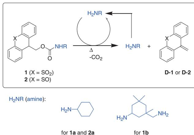
**Scheme 1.** Autocatalytic fragmentation of BAs **1** and **2** having oxidized thioxanthene moieties.
