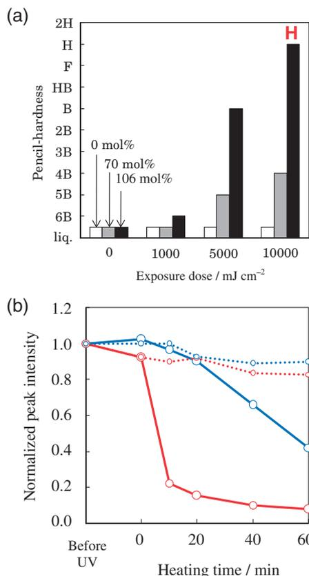
**Figure 7.** (a) Pencil-hardness of EX-622 coating films containing 10 mol % of **4** and 0, 70, or 106 mol % of **1b** as a function of exposure dose of 365 nm-light. Postbaking was performed at 60 °C for 20 min. (b) Changes in peak intensities of carbonyl moieties of **1b** (red) and epoxy moieties of the resin (blue) in FT-IR measurements as a function of heating time with (solid line) and without (dotted line) 5000  $\text{mJ cm}^{-2}$  of UV irradiation. Postbaking was performed at 60 °C.
