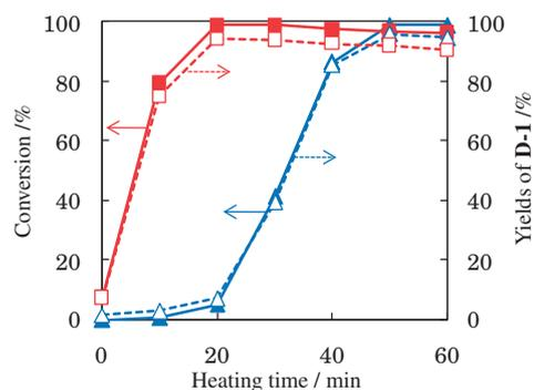
**Figure 1.** The consumption of **1a** (conversion, closed symbols) and the formation of **D-1** (yield, open symbols) as a function of heating time in the presence (red) and the absence (blue) of 13 mM of piperidine in 1,4-dioxane-*d*<sub>8</sub> at 100 °C.
