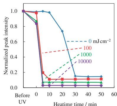
**Figure 3.** The consumption of **1a** as a function of heating time in polystyrene films containing 10 wt % of PBG **3** after 0–10000  $\text{mJ cm}^{-2}$  of UV irradiation followed by postbaking at 60 °C.
