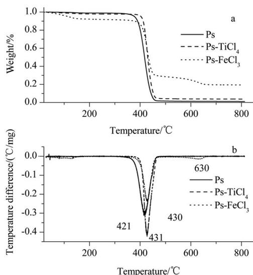
**Figure 1** TGA thermograms for Ps, Ps-TiCl<sub>4</sub> and Ps-FeCl<sub>3</sub>.
