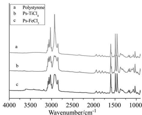
**Figure 3** FTIR spectra of Ps, Ps-TiCl<sub>4</sub> and Ps-FeCl<sub>3</sub>.
