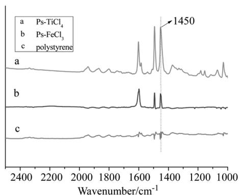
**Figure 4** Pyridine-adsorbed FTIR of Ps, Ps-TiCl<sub>4</sub> and Ps-FeCl<sub>3</sub>.
