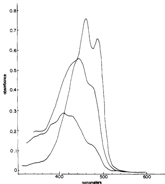
Figure 1. UV spectra of the thermal degradation mixture of  $\beta,\beta$ -carotene: (1) absorbance = 0.77, 30 min at 170 °C; (2) absorbance = 0.56, 180 min at 170 °C; (3) absorbance = 0.29, 371 min at 170 °C.
