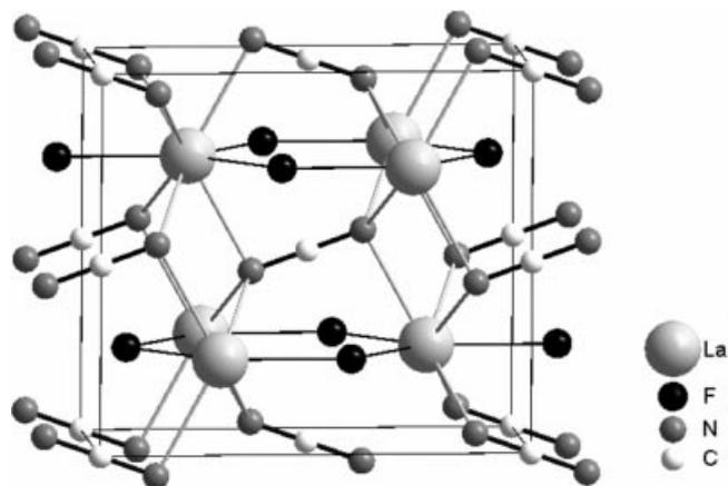
**Figure 1.** View along the approximate [100] direction of the crystal structure of  $\text{LaF}(\text{CN}_2)$ .
