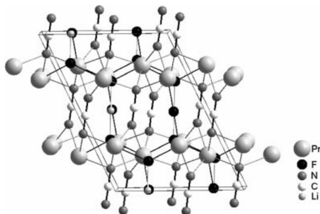
**Figure 4.** View along the approximate  $[010]$  direction of the crystal structure of  $\text{LiPr}_2\text{F}_3(\text{CN}_2)_2$ .
