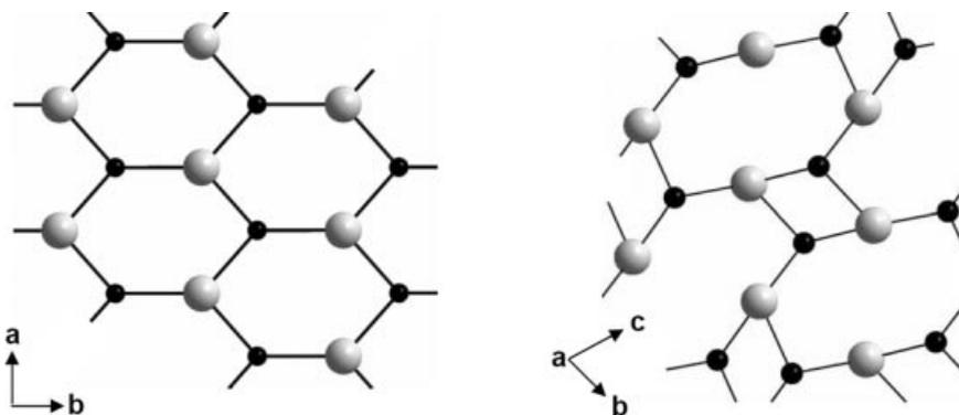
**Figure 2.** Section of [LaF] layers in the structures of  $\text{LaF}(\text{CN}_2)$  (left) and  $\text{LiPr}_2\text{F}_3(\text{CN}_2)_2$  (right). Note that the layer at right is not fully planar.
