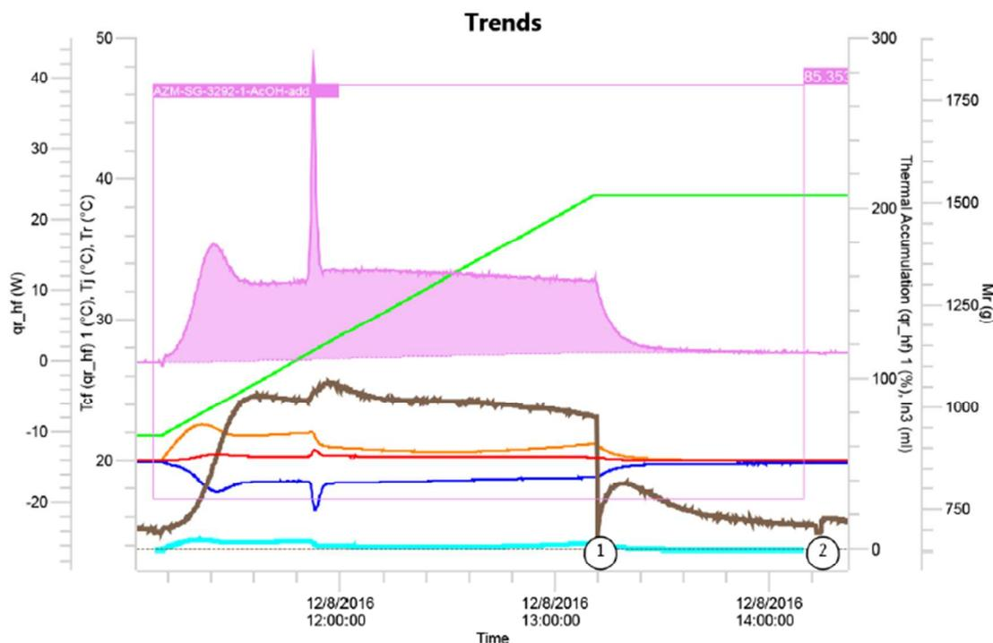
Figure 3: Reaction calorimetry test on benzylvanillin. 587 g of **2** (23.8 w/w %) was dosed into the reaction mixture at 20 °C during 2 h. The mixture was stirred for an additional 1h at the same temperature. Heat generation in pink. The sharp peak is caused by precipitation of the product.
