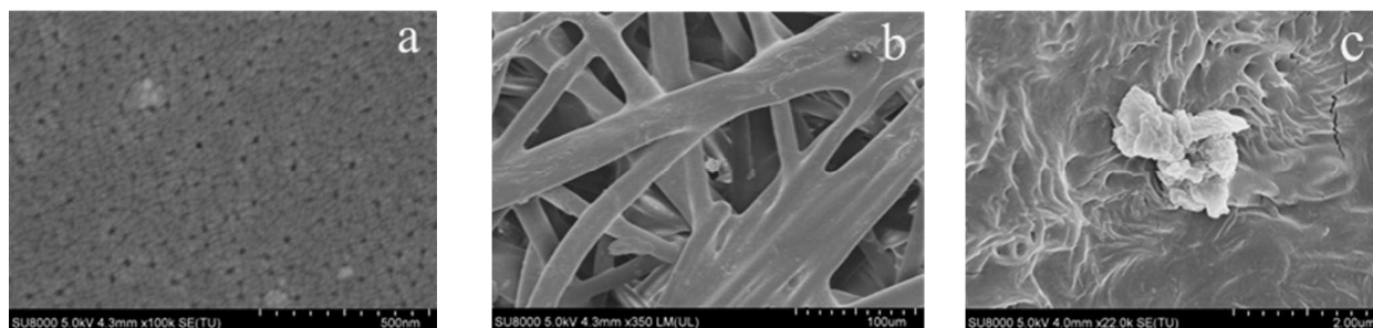
Figure 2. SEM images of (a) Membrane skin layer (regenerated cellulose); (b) Support layer (nonwoven polypropylene); (c) View of support layer after enzyme immobilization.
