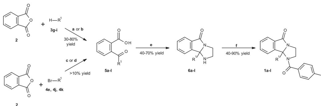
Scheme 1. Reagents and conditions: (a) AlCl<sub>3</sub>, 90–110 °C, 3 to 5 h; (b) AlCl<sub>3</sub>, 0 °C to rt, 16 h; (c) **4e**, Mg, cat. I<sub>2</sub>, 40 °C then rt, 1 h followed by **2**, –60 °C, 1.5 h then rt, 1.5 h; (d) **4j** or **4k**, *n*-BuLi, Et<sub>2</sub>O, –78 °C, 30 min followed by **2**, THF, –78 °C, 1 h then rt; (e) ethylenediamine, toluene or xylenes, Dean–Stark, reflux, 2–5 h; (f) 4-fluorobenzoyl chloride, pyridine, 0 °C to rt.
