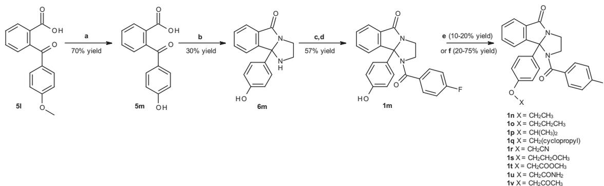
**Scheme 2.** Reagents and conditions: (a) pyridine hydrochloride, 195 °C, 5 h; (b) ethylenediamine, xylenes, Dean–Stark, reflux, 7 h; (c) 4-fluorobenzoyl chloride, pyridine, 0 °C to rt; (d) 1 M NaOH (aq.), MeOH, rt, 30 min; (e) XOH, PS-PPh<sub>3</sub>, DEAD, THF, 0 °C to rt; (f) XBr or XCl, K<sub>2</sub>CO<sub>3</sub>, acetone, reflux.
