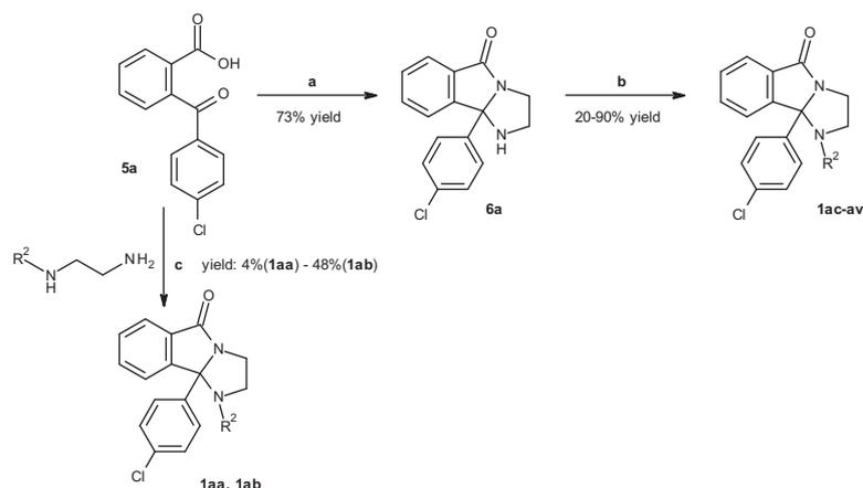
**Scheme 4.** Reagents and conditions: (a) ethylenediamine, toluene, Dean–Stark, reflux, 5 h; (b) acid chloride or isocyanate, pyridine, 0 °C to rt; (c) xylenes, Dean–Stark, reflux.
