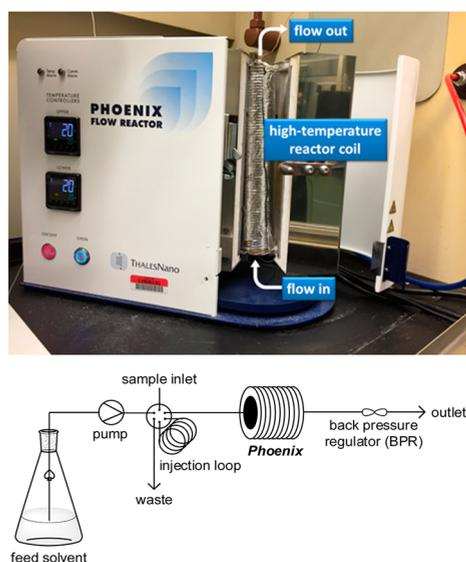
Figure 1. Schematic of the high-temperature Phoenix flow reactor.
