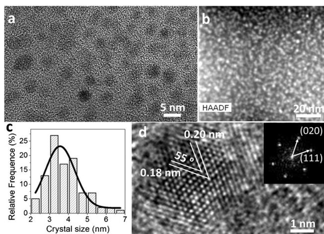
**Figure 1.** a) TEM image of nickel nanocrystals. b) HAADF image of nickel nanocrystals in large-area view. White dots in the HAADF image are nickel nanocrystals. c) Crystal size distribution. d) High-resolution TEM image of a nanocrystal. Inset: corresponding FFT image.
