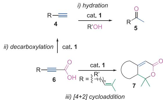
**Figure 1.** Catalytic reactions of alkynes and oxygen atom featuring Au(DPB<sup>R</sup>)X 1.
