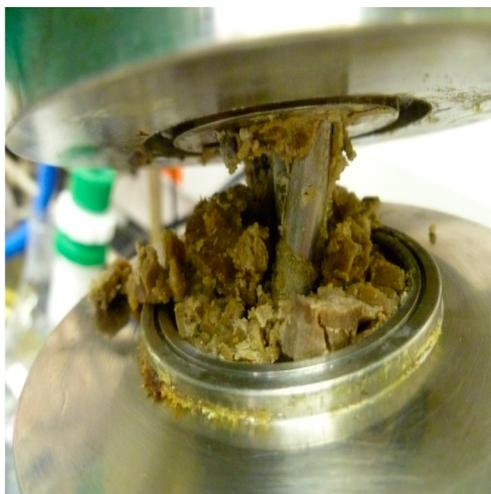
Figure 3. Twenty-five mL reactor after fouling, running with 4.2 L/kg of toluene.
