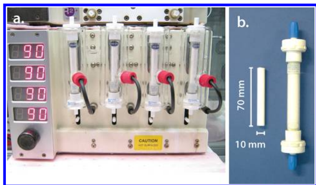
Figure 1. (a) A batch of monoliths undergoing the curing process in a convection heater. (b) Prepared monolithic reagents, removed from and within the glass column reactor.
