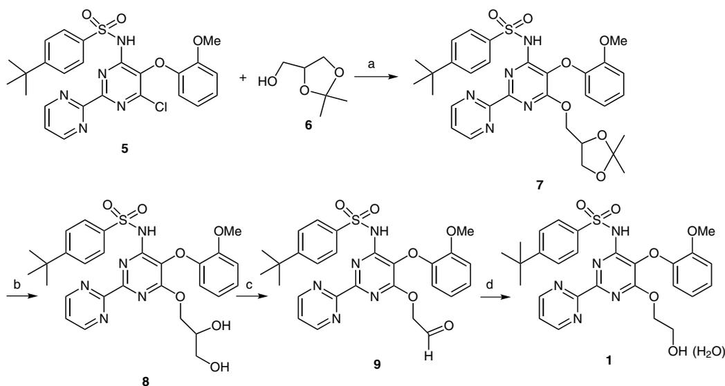
**Scheme 1** Alternate synthesis of bosentan monohydrate (**1**). *Reagents and conditions:* (a) NaOH, MeCN, 80–85 °C, 12 h; (b) 2 M HCl, MeCN, r.t., 5 h; (c) NaIO<sub>4</sub>, acetone, H<sub>2</sub>O, 0 °C to r.t., 3 h; (d) NaBH<sub>4</sub>, MeOH, 0 °C to r.t., 4 h.
