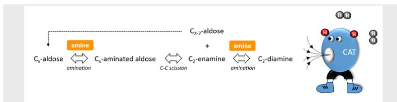
Reductive aminolysis of carbohydrates to short diamines and aminoalcohols in presence of heterogeneous metal catalysis is effective at low temperature thanks to the facilitative effect of the amine reagent on the carbon-carbon scission.
