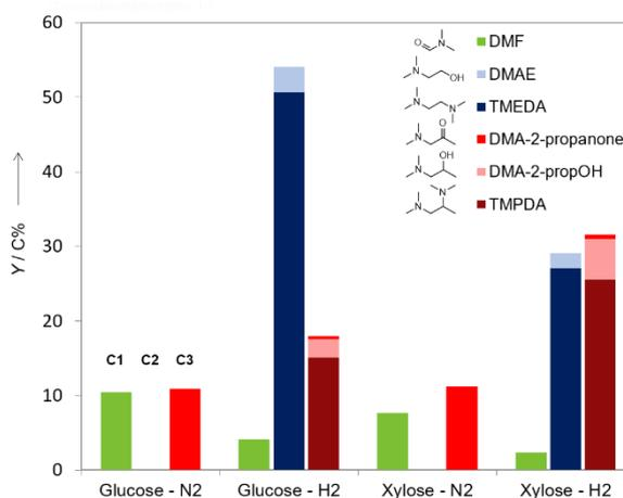
**Figure 1.** Product distribution for glucose and xylose aminolysis obtained after 1 h (full sugar conversion) at 398 K with Ru/C under i) atmospheric N<sub>2</sub> pressure (0.1 MPa) and ii) elevated H<sub>2</sub> pressure (7.5 MPa).
