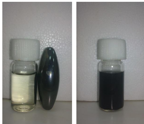
Fig. 11. MPNC are attracted to the wall of the vial in presence of a magnet.
