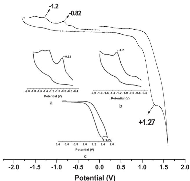
**Fig. 1.** Cyclic voltammogram of [(Mo<sup>VI</sup>O<sub>2</sub>)<sub>2</sub>L] (**1**) in DMSO showing (a) reduction of (Mo(VI)→Mo(V)), (b) reduction of (Mo(V)→Mo(IV)) and (c) oxidation of ligand.
