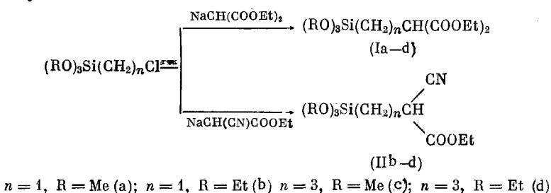
The (triethoxysilyl)alkylation of sodium ethyl cyanoacetate gives bis[(triethoxysilyl)-alkyl]cyanoacetates  $[(EtO_3)_3Si(CH_2)_n]_2C(CN)CO_2Et$  ( $n = 1$  (III) and  $n = 3$  (IV)) in addition to the monosubstitution products (IIb) and (IId).
