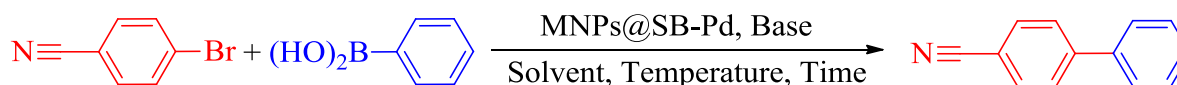
Scheme 2. Suzuki-Miyaura cross-coupling reaction between 4-bromobenzonitrile with phenylboronic acid in the presence of MNPs@SB-Pd nanomagnetic catalyst.
