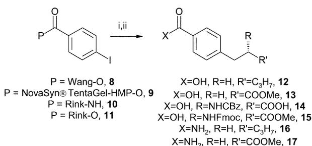
**Scheme 1** Reagents and conditions: i, organozinc 1–4 in THF (3 equiv.), Pd<sub>2</sub>(dba)<sub>3</sub> (10 mol%), P(*o*-tolyl)<sub>3</sub> (40 mol%), room temp., 16 h; ii, TFA–dichloromethane, 1 h.
