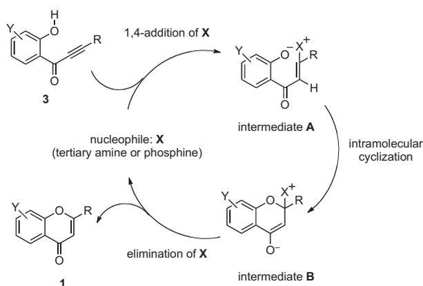
Scheme 1. A catalytic cycle in the regioselective synthesis of **1** from **3**.
