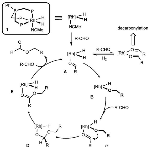
Scheme 2. Proposed mechanism for the dimerization of aldehydes catalyzed by **1**.
