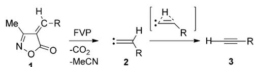
**Scheme 1.** Synthesis of acetylenes **3** by FVP of isoxazolones **1**.
