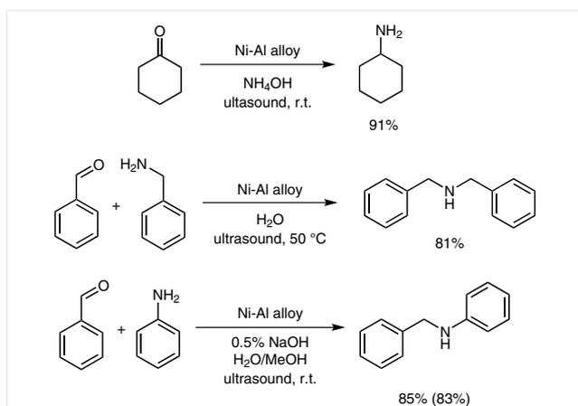
**Scheme 2** Scale-up of reductive amination reactions. Reactions were carried out on a 5 mmol scale using the corresponding conditions (see Tables 2–4). Yield in parentheses corresponds to isolated yield.
