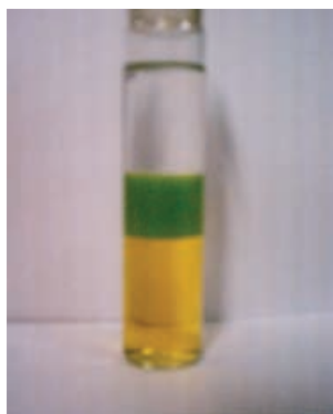
Figure 1. Top phase: organic phase, middle phase: catalyst-rich phase, bottom phase: aqueous phase.
