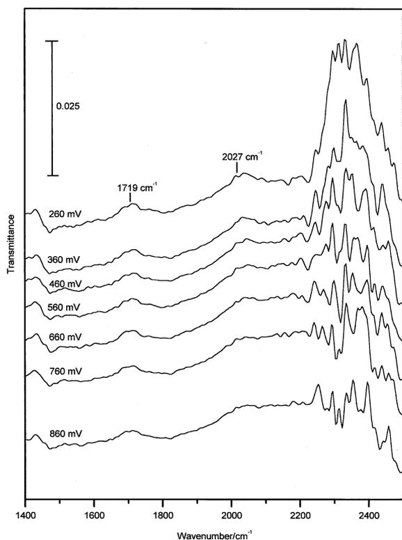
Fig. 3. 'In situ' LPS-FTIR spectra from a platinumized Pt in 0.5 M  $\text{HClO}_4$  with  $\text{D}_2\text{O}$ ;  $\text{CH}_4$  adsorbed at 0.26 V for 1 h (referenced to reflectance at 1.46 V).
