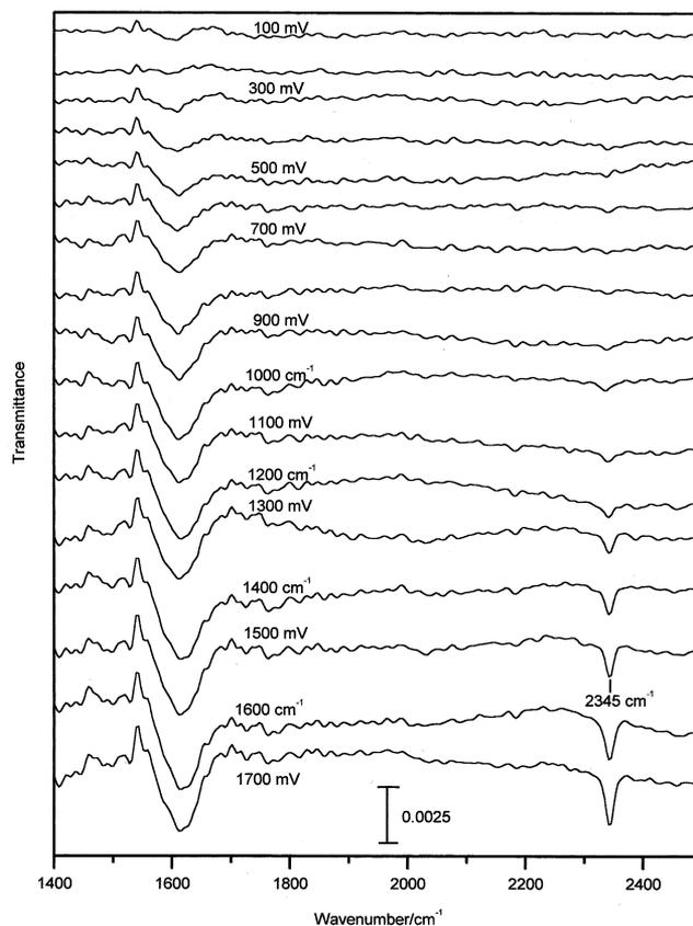
Fig. 8. 'In situ' LPS-FTIR spectra from a smooth Au electrode;  $\text{CH}_4$  adsorbed at 0.0 V for 1 h (referenced to reflectance at 0.0 V).
