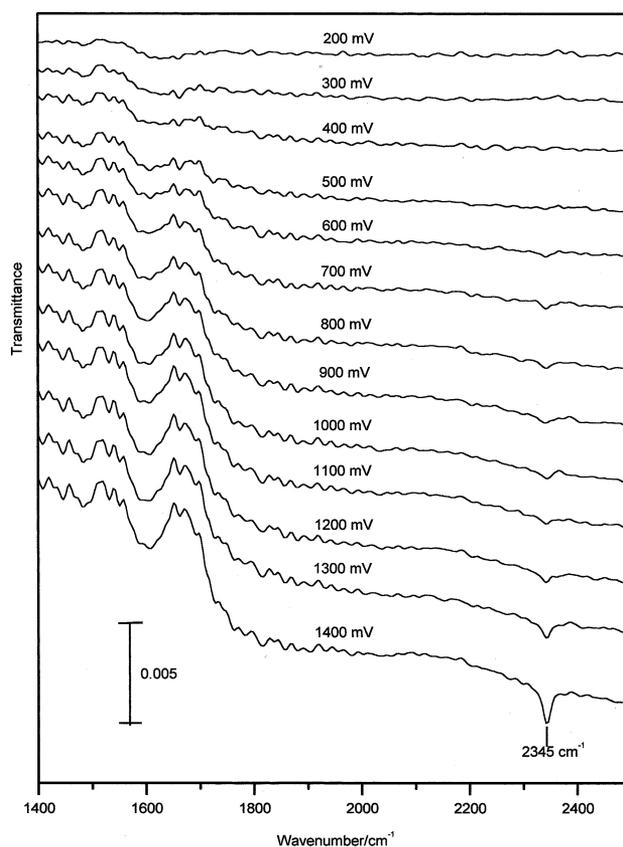
Fig. 6. 'In situ' PDIR spectra from a Ru disc electrode;  $\text{CH}_4$  adsorbed at 0.1 V for 2 h (referenced to reflectance at 0.1 V).
