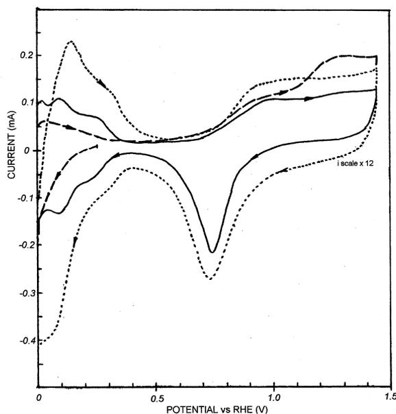
Fig. 1. Cyclic voltammograms of Pt in 0.5 M  $\text{HClO}_4$  deaerated solution (solid line) and after bubbling  $\text{CH}_4$  through the solution for 2 h (broken line) at 0.26 V; cyclic voltammogram of platinized Pt (dotted line); scan rate = 100 mV/s.
