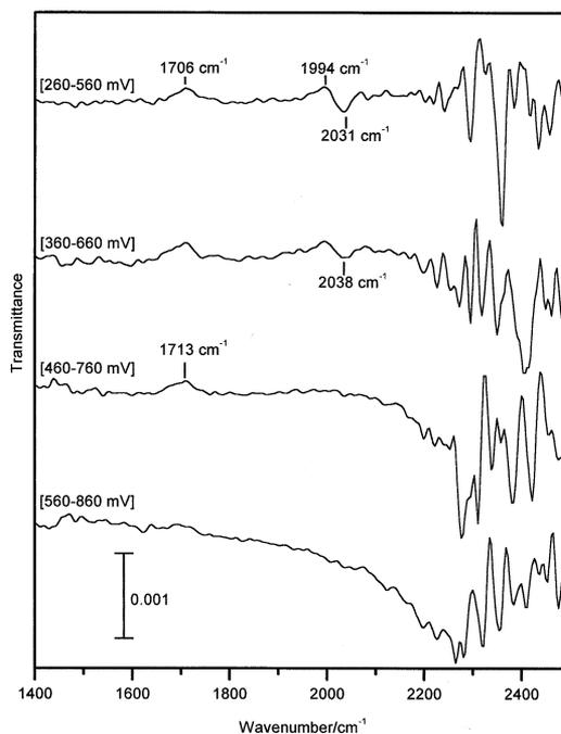
Fig. 4. 'In situ' IR spectra from a platinumized Pt in 0.5 M  $\text{HClO}_4$  with  $\text{D}_2\text{O}$  obtained by the SNIFTIRS technique;  $\text{CH}_4$  adsorbed at 0.26 V for 2 h; modulation potentials indicated in brackets.
