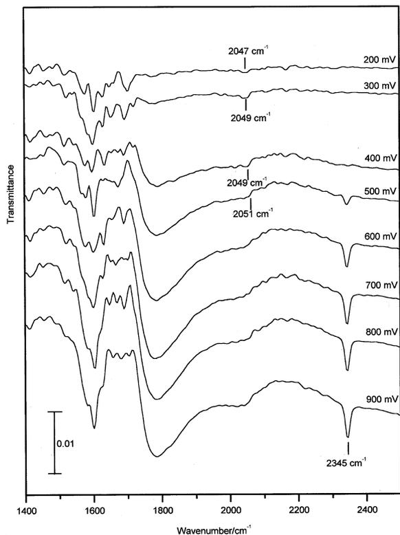
Fig. 7. 'In situ' PDIR spectra from a ruthenized Ru electrode;  $\text{CH}_4$  adsorbed at 0.1 V for 2 h (referenced to reflectance at 0.1 V).
