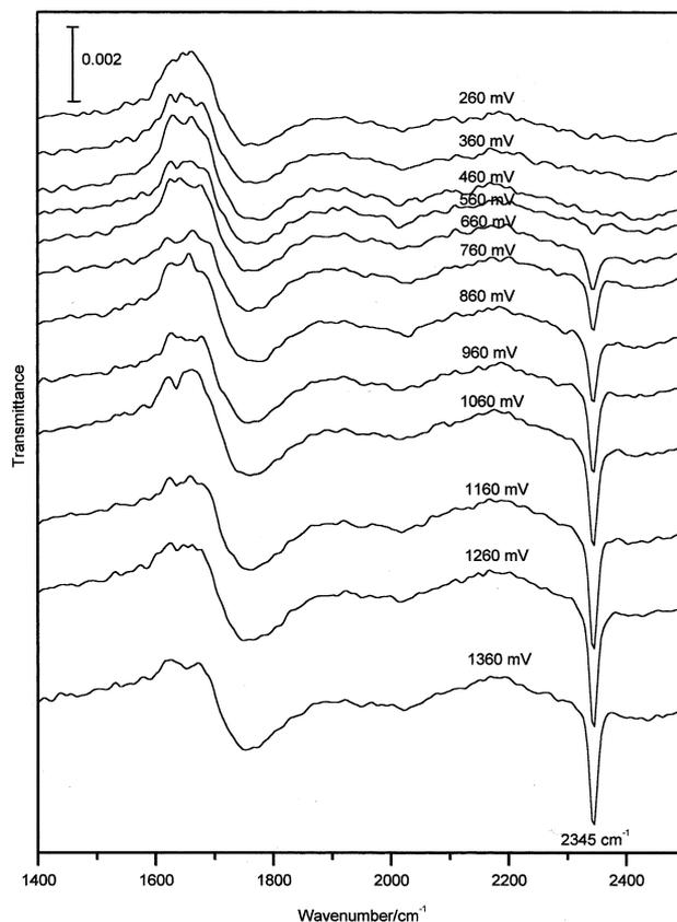
Fig. 2. 'In situ' LPS-FTIR spectra from a Pt disc electrode as a function of potential following adsorption of  $\text{CH}_4$  at 0.16 V for 45 min (referenced to reflectance at 0.16 V).
