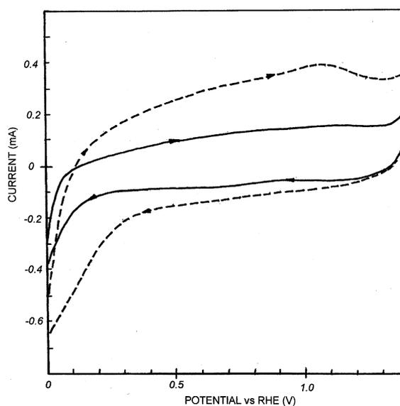
Fig. 5. Cyclic voltammograms of a polycrystalline Ru disc electrode (solid line) and a ruthenized Ru electrode (broken line) in 0.5 M  $\text{HClO}_4$  solution; scan rate = 100 mV/s.
