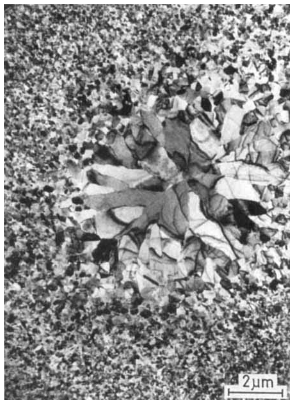
Fig. 1. Ordered and disordered \text{AlNi}_3 crystal plates which typically grow in laser pulse molten 1 Al: 3 Ni films within 4 \mu\text{s} (laser pulse 20 ns FWHM, \approx 1 \mu\text{J} )
