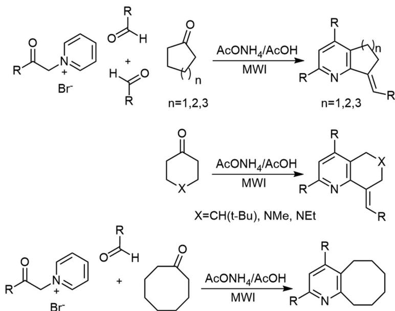
**Scheme 1.** Microwave assisted synthesis of annulated pyridines.
